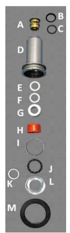
REBUILDING POT BEARING HOUSINGS: The used assembly is disassembled, cleaned and inspected. Epic **always** replaces the felt sealing washer (E), upper needle bearing (G), nylon spacer bushing (H), lower outer race (I), and bearing cage, polyamide (J). Any static parts that show wear or faults are also replaced. The rebuilt assembly is lubricated with Kluber synthetic grease.
